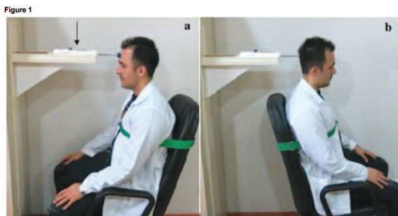
Measurement of isometric neck flexion (a) and extension (b) strength. Arrow shows the placement of the force gauge.
